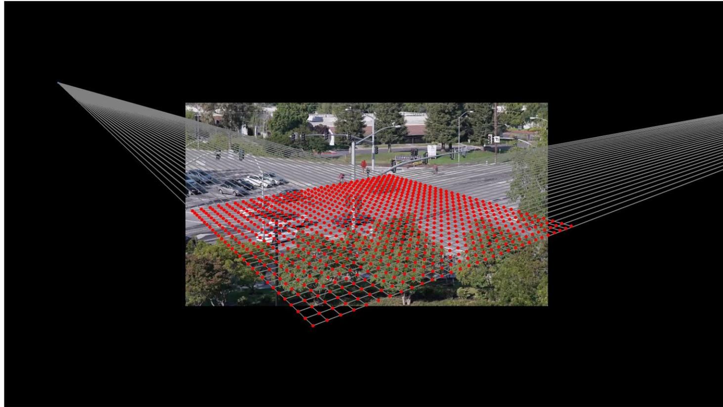
Visualization of estimated ground plane: The red dots form a (30 m \* 30 m) 3D grid on the ground plane projected to 2D space
