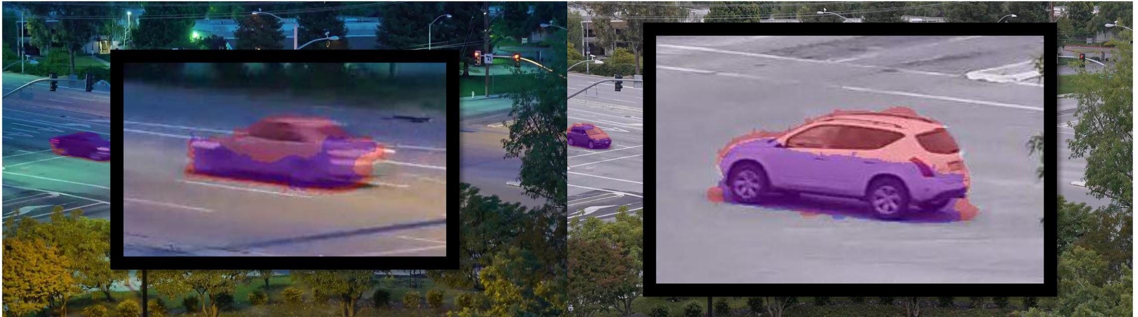
Blue: preliminary segmentation from SuBSENSE with shadow detection
